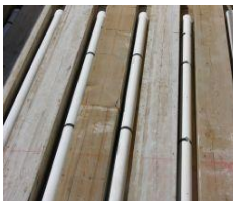
The composting bins were located at the District of Kent wastewater treatment plant. They contained aeration pipes to optimize oxygen supply and temperature.
