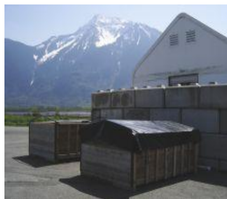
After placing the composting material in the bins, it was covered with a layer of screened compost overs that serve as odor barrier and with a frame and tarpaulin cover for protection.
